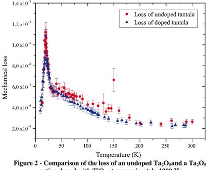
coating doped with TiO<sub>2</sub> at approximately 1000 Hz. (doping\_comparison\_undoped\_1kHz.txt, doping\_comparison\_14\_5%\_1kHz.txt)
