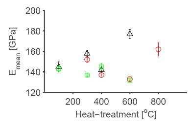
Figure 6 - Mean Young's moduli of tantala samples measured on silica substrates, plotted for different heat-treatments. Red circles are pure tantala, green squares are 25% titania-doped tantala, and black triangles are 55% titania-doped tantala.
