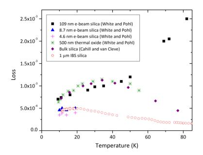
Figure 3 - Comparison of the mechanical dissipation of ion-beam sputtered silica with bulk silica, e-beam evaporated silica and thermal oxide grown on silicon. (IBS\_Silica\_7kHz.txt)
