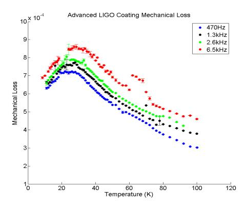
Figure 4 – Mechanical loss of an Advanced LIGO silica/titania-doped tantala coating on a silicon cantilever.
