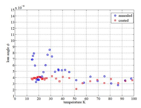
Figure 5 – Mechanical loss of an as-deposited (coated) and a 500 °C heat treated (annealed) multilayer silica/tantala coatings on sapphire disks.
