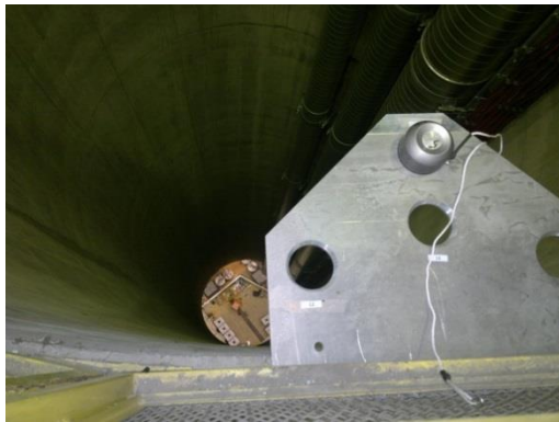
Figure 2: Adapted Taylor-Hobson sphere and forced centring plate above the CERN ECA4 shaft
