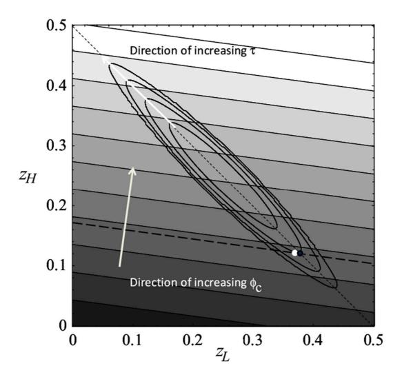
**Figure 3** – Contours of constant reflectance and contours of constant Brownian noise in a 5 - doublets coating, as functions of the optical thickness of the low and high index layers.
