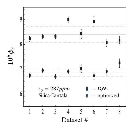
**Figure 6** – Coating loss angle of QWL and optimized coating measured at TNI (A. Villar et al., 2010)
