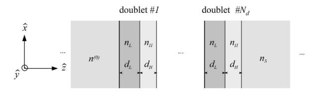
**Figure 2** – Stacked – doublet coating geometry, showing the relevant notation for the layer thicknesses and refraction indexes
