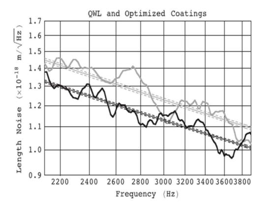
Figure 5 – Smoothed spectra of QWL (gray) and optimized (black) coating measured at TNI. Rellated fits (solid lines) and confidence intervals (dashed lines) also shown (A. Villar et al., 2010)
