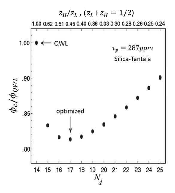
**Figure 4** – Coating loss angle of iso - reflective coatings consisting of a different number of Bragg doublets, with different thickness ratios  $z_H/z_L$ .
