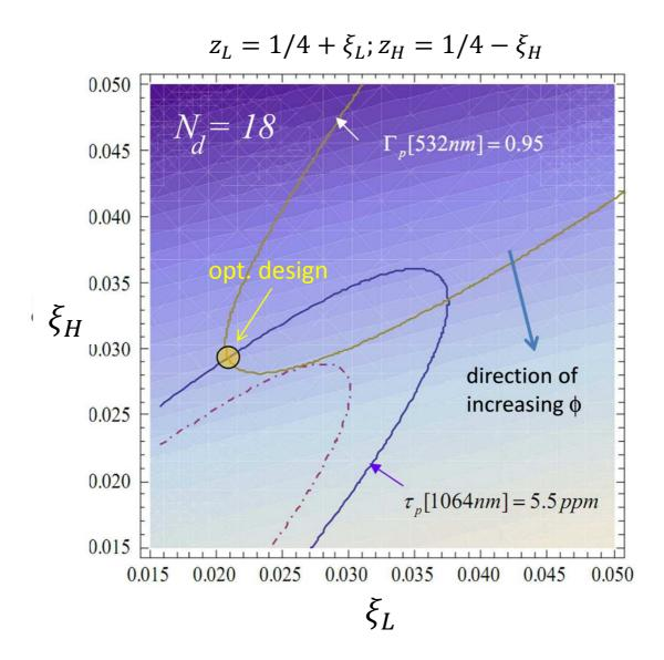
Figure 7 – Stacked doublet dichroic mirror. Constant reflectance contours and constant noise density vs. doublet thickness (M. Principe et al., LIGO G1000380).
