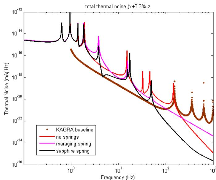
Figure 5. Thermal noise estimate with springs at the final stage (for a single test mass)
