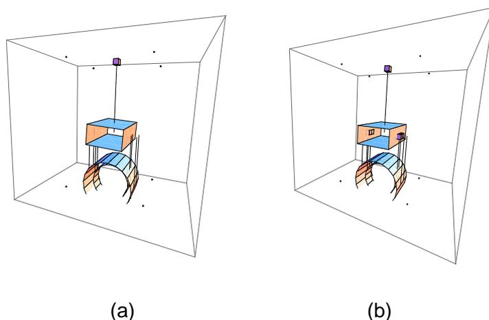
Figure 1. (a) Mathematica model configuration without final stage springs (b) Mathematica model configuration with final stage springs
