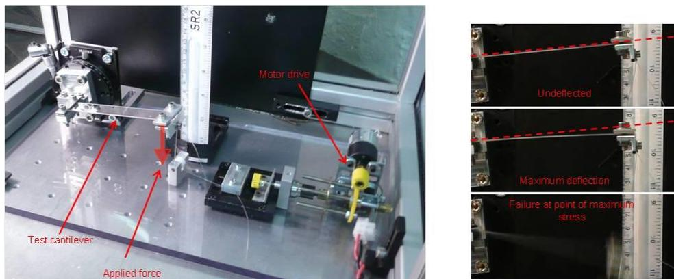
Figure 7. Cantilever spring strength testing apparatus
