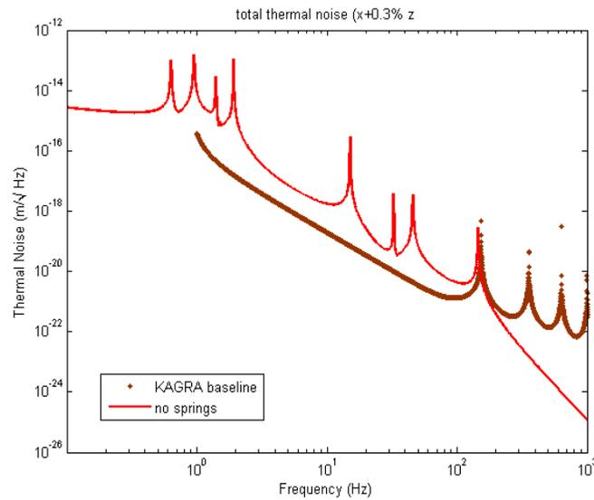
Figure 2. Thermal noise estimate without springs at the final stage (for a single test mass)
