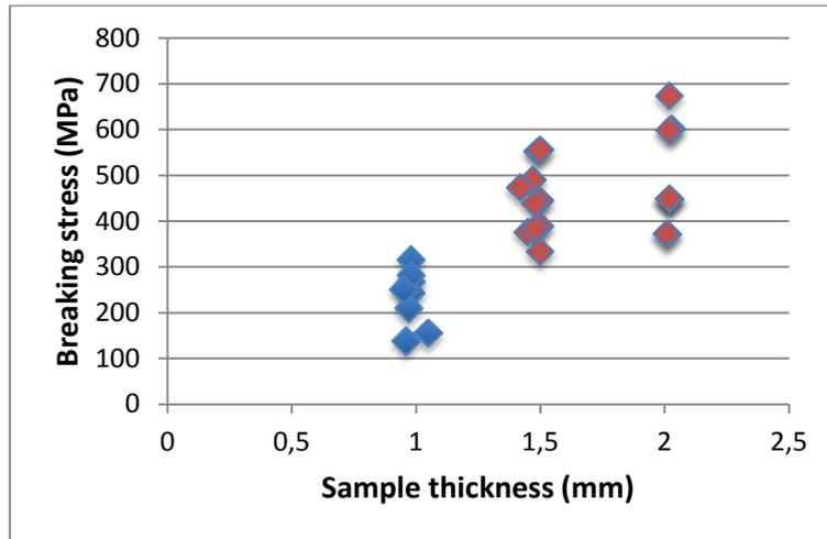
Figure 8. Breaking stress of sapphire slides at maximum deflection.
