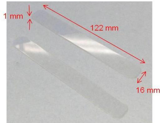
Figure 6. IMPEX sapphire slide
