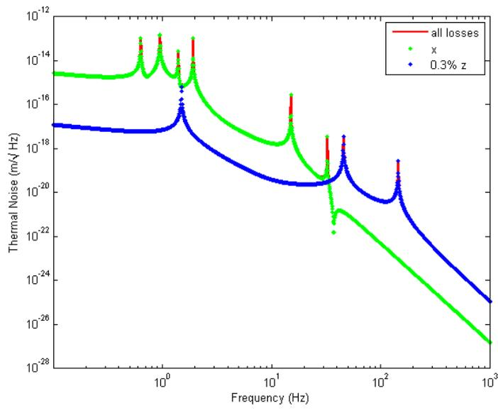
Figure 4. Thermal noise contribution from the recoil mass wires
