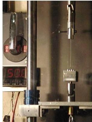
Figure 11a. IMPEX nail end fibre clamping jig b. IMPEX nail end fibre on tensile strength testing machine, just before point of failure (fracture at nail end) at 50.3 kg.
