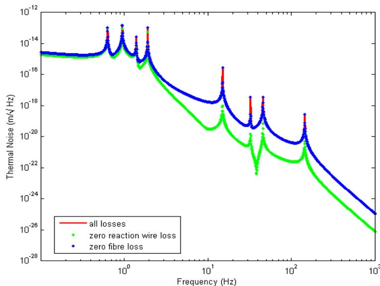
Figure 3. Thermal noise estimate without springs and for the different loss terms set to zero
