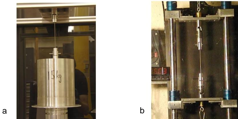
Figure 9a. Moltech fibre hanging 15 kg strength test mass b. Moltech fibre on tensile strength testing machine, at point of failure (in the clamp) at 60.3 kg.
