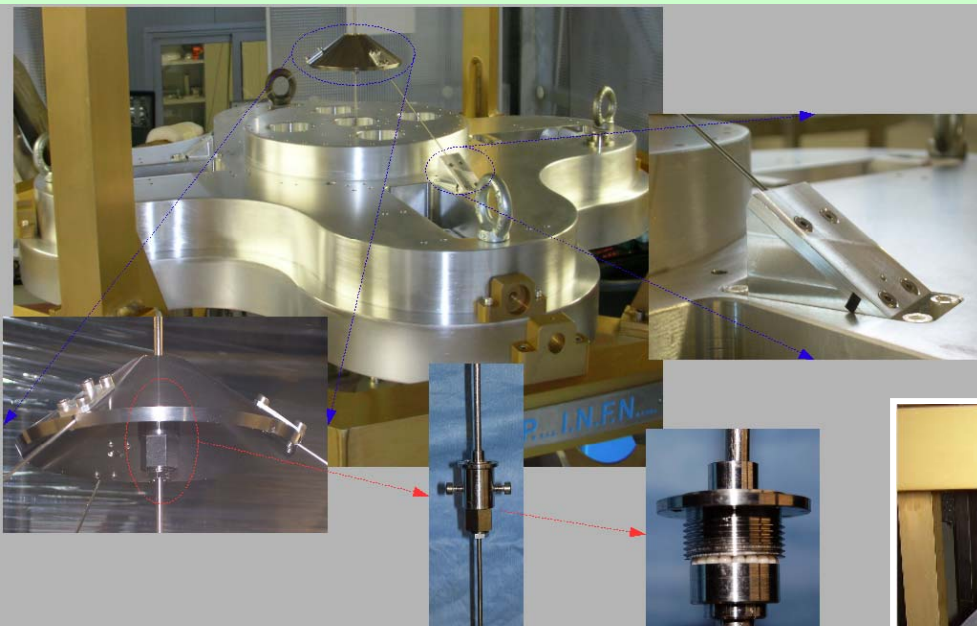
Suspension System of the payload and MRM
