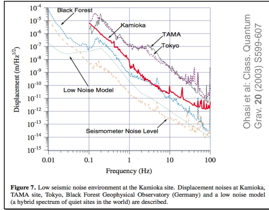
Figure 7. Low seismic noise environment at the Kamioka site. Displacement noises at Kamioka, TAMA site, Tokyo, Black Forest Geophysical Observatory (Germany) and a low noise model (a hybrid spectrum of quiet sites in the world) are described.
