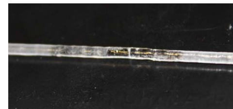
Sapphire jointed at 80W
