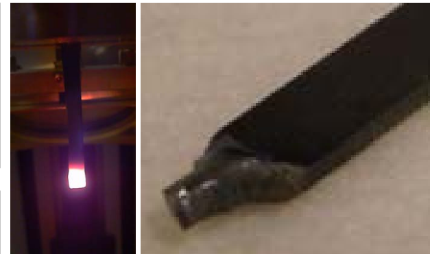
Silicon melted at 90W in air
