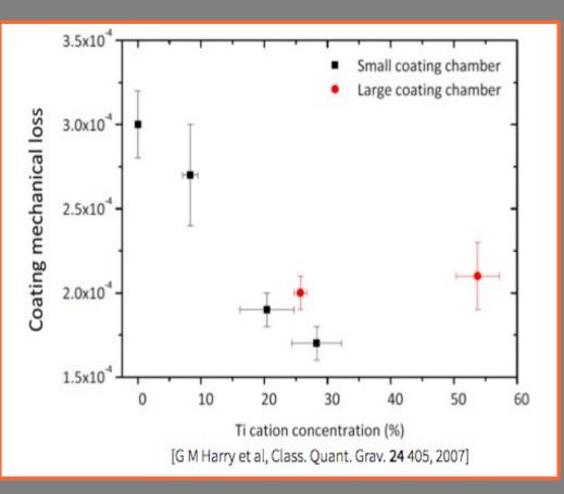
TiO<sub>2</sub> doping: reduces the mechanical dissipations
