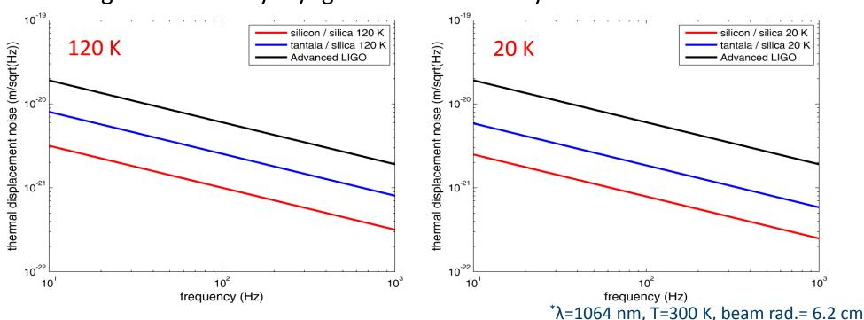
Coating loss limited by cryogenic loss of silica layers
