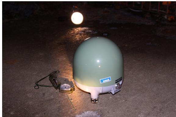
Figure 2: The Trillium 240 simply placed on a concrete platform, aligned by using a compass.
