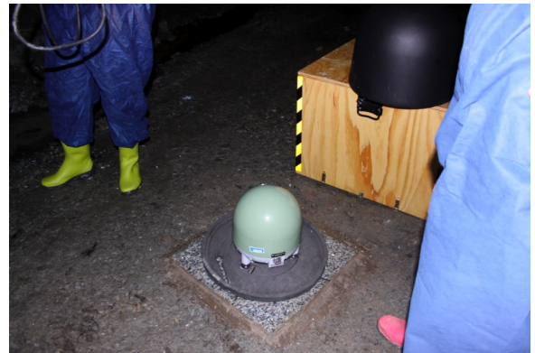
Figure 3: A granite tile is attached and leveled on the ground through a mixture of concrete and sand. After the concrete hardening the seismometer is placed on it.
