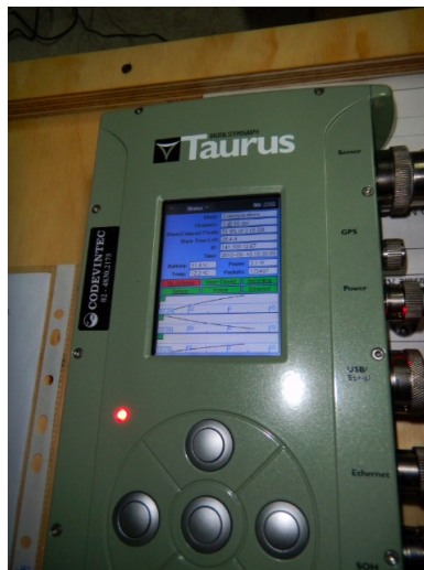
Figure 1: The Taurus acquisition system, remotely controllable, is connected to a 12V battery and to the Trillium seismometer.
