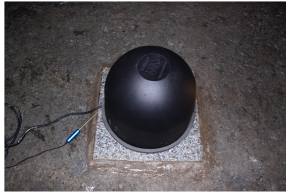
Figure 4: The insulating cover includes a foam base gasket and a rigid form-fitting cover with form features matched to the Trillium 240.
