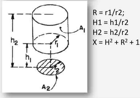
Radiation from int. surface of cylnder of radius  $r_1$  to disk of radius  $r_2$ , were  $r_2 < r_1$ ; disk is perpendicular to axis of cylinder, and axis passes trough center of disk.
