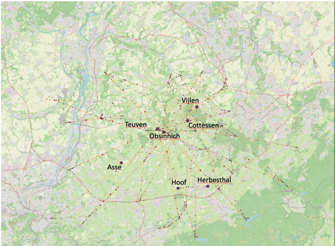
Figure 4c: Network of 700 noise sensors set up in passive seismic mode to develop a regional surface noise model, and to supplement sub-surface noise measurements to develop a regional subsurface model.
