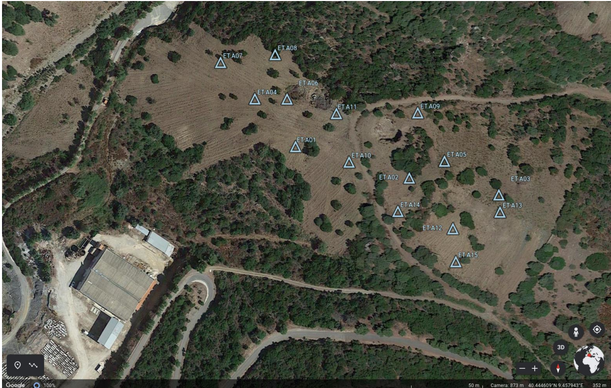
Fig. 18. Geometry of the surface seismic array deployed at Sos Enattos on January 2021.
